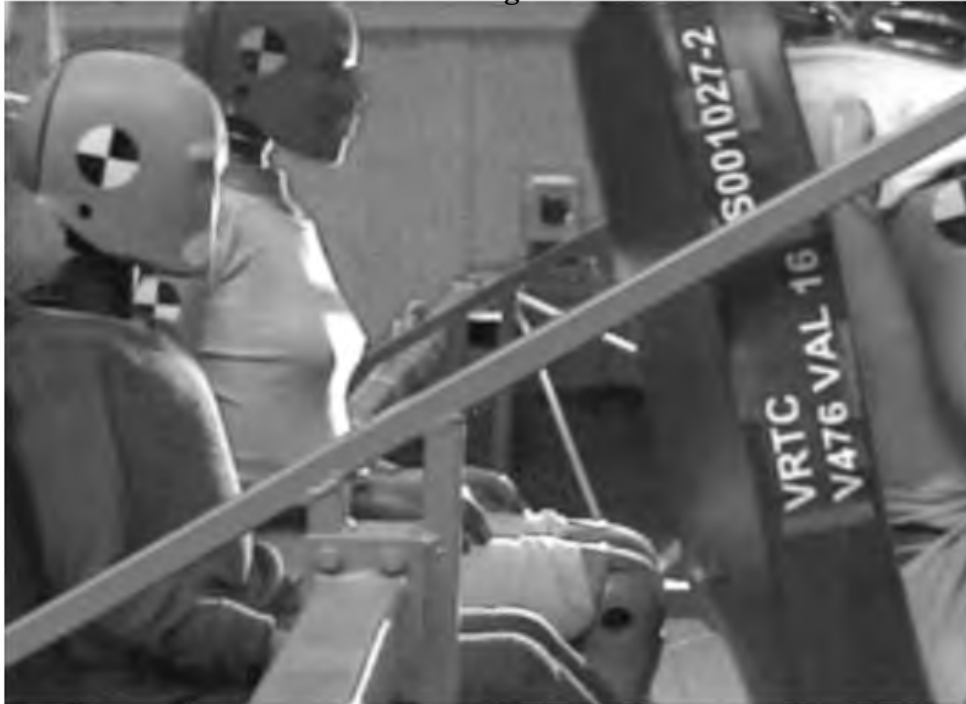
Figure 16. Initial Position of the 6-year-old and 5th Percentile Female Dummies
