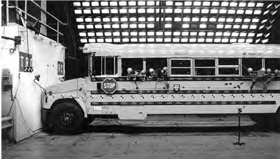
Figure 1. Pre-Crash Photograph of Frontal School Bus Test.
