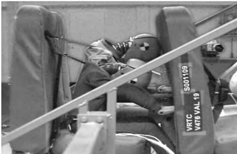
Figure 21. Lap/Shoulder Belt Test at Maximum Neck Flexion
