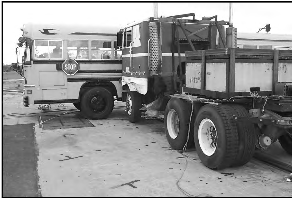
Figure 7. Pre-Test Photograph of Side Impact School Bus Crash Showing Bullet Truck
