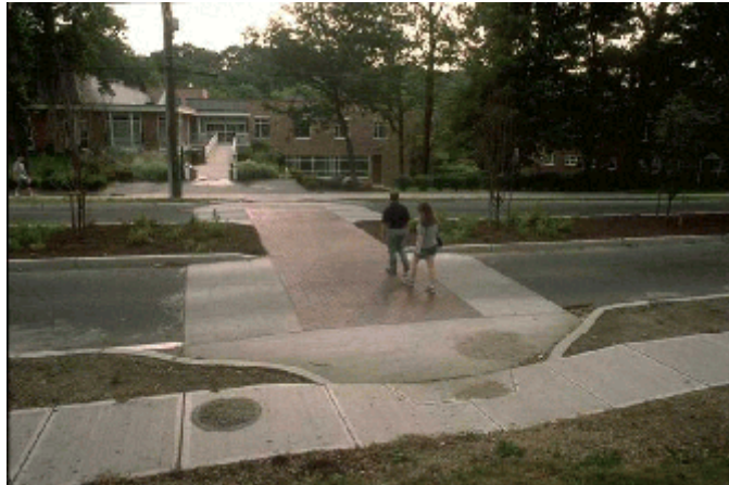
Figure 13. Raised crosswalks can control vehicle speeds on local streets at pedestrian crossings.
