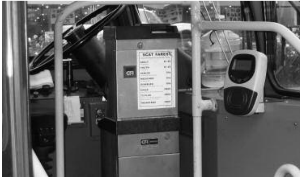
Figure 8 - Smart Card Reader and Fare Box
