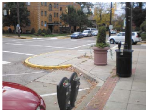
Photo 9 - An example of sidewalk bulb-outs, which provide greater visibility for both motorists and pedestrians, and also shorten the distance of exposure for pedestrians using the crosswalk.
