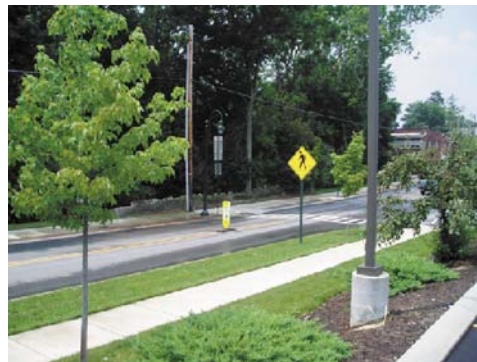
Photo 8 - Example of in-street pedestrian signs and crosswalk signs used together to emphasize pedestrian crossing location
