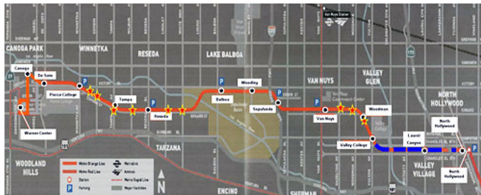
Metro Orange Line pavement repair map: Blue sections represent full-depth pavement replacement; stars mark the intersections where grind and overlay repairs will be undertaken in phase 2.
