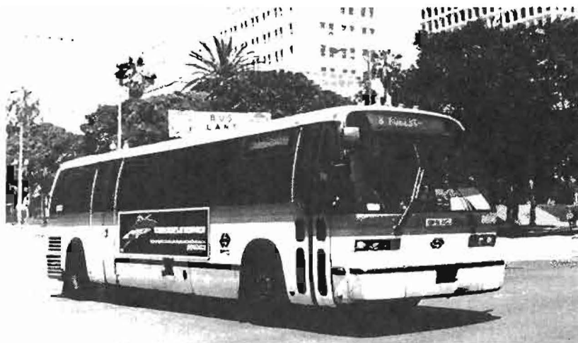
940 of these new GM Advanced Design buses were placed into service by RTD during an eight-month period ending August 4, 1981. At a cost of $141,000, each bus seats 43 passengers and can accommodate two persons in wheelchairs.
