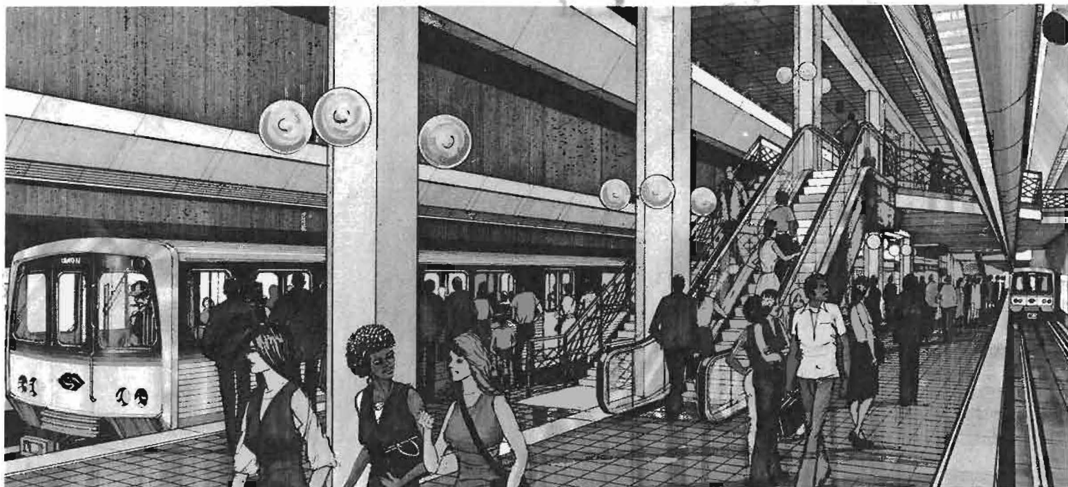
Rendering of Metro Rail station at platform level. The 450-foot platforms accommodate up to a six-car train. Escalators, stairs and elevators are included in the design of each RTD station.
