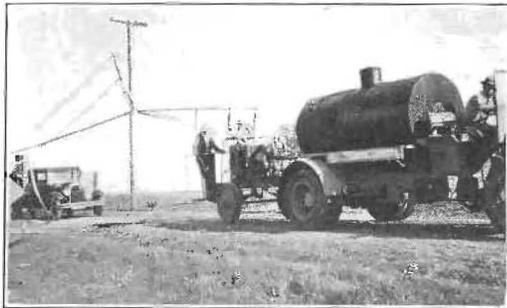
Weed spraying unit attached to 1000-pound truck.
