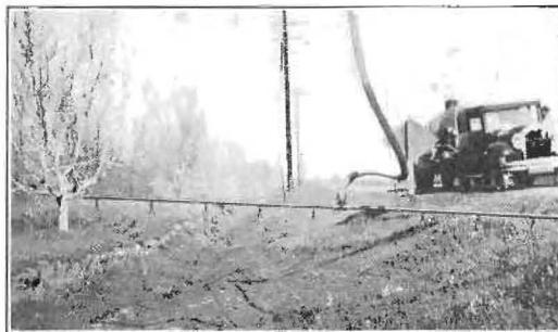
Spraying arm in working position.
