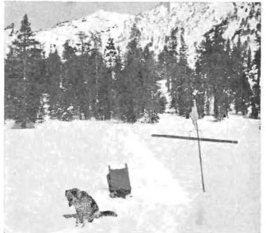
**TYPICAL SNOW COURSE** showing sampling tube and scales. The scales record water content of snow in tube. In foreground is surveyor's dog companion and heavy pack.
