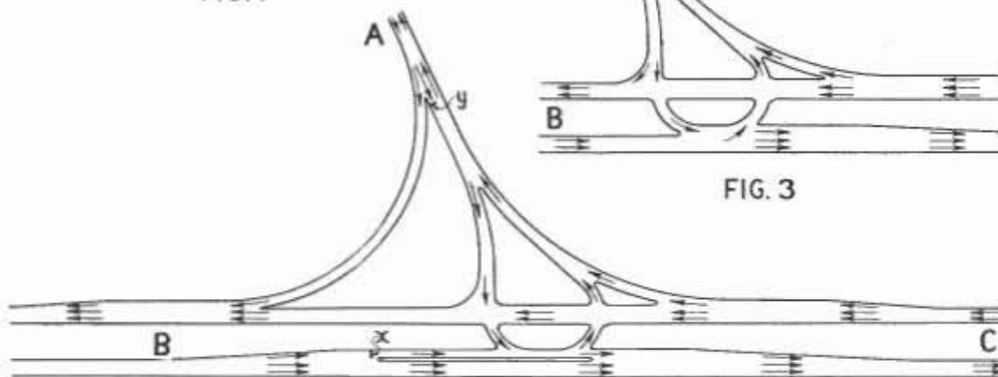
Illustrating stages in the expansion of the simple "Y" type intersection at grade to keep pace with increasing traffic volume.
