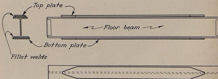
PLATE METHOD OF STRENGTHENING FLOOR BEAMS
