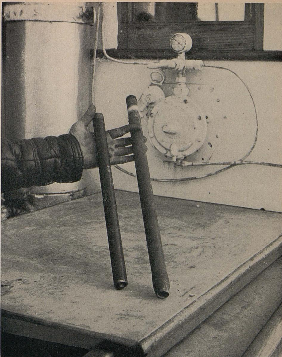
Sampler tips. Cutting point on right used for hard material
