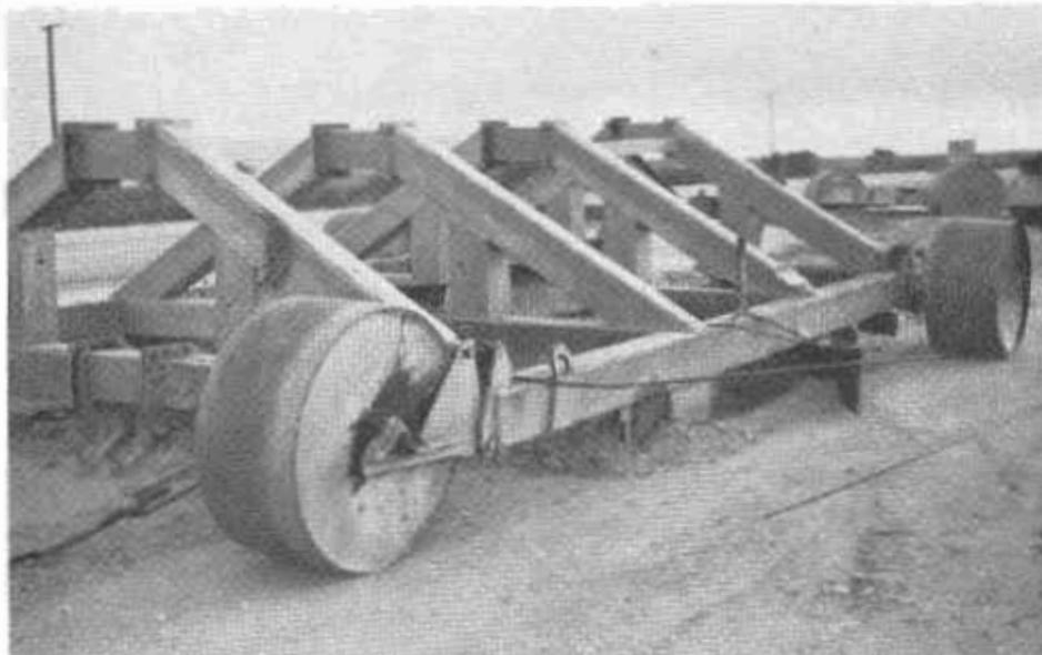
Towed frame developed by a California contractor to scarify and windrow in-place material preparatory to cement treatment. Equipment can be adapted to work from side form by replacing wide base steel wheels with narrower flanged wheels.
