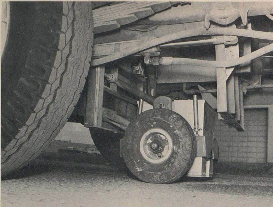
FIGURE 4—The moisture unit lowered into logging position.
