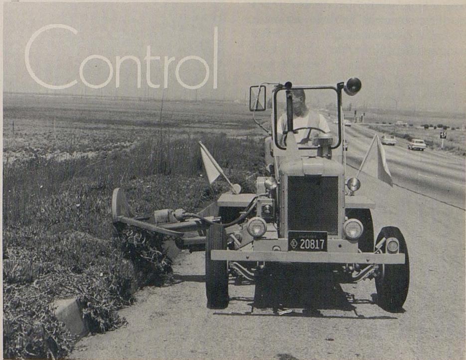
*The newly developed ice plant cutter, with blade encased for safety, trims vegetation with a minimum of manpower and traffic disturbance.*
