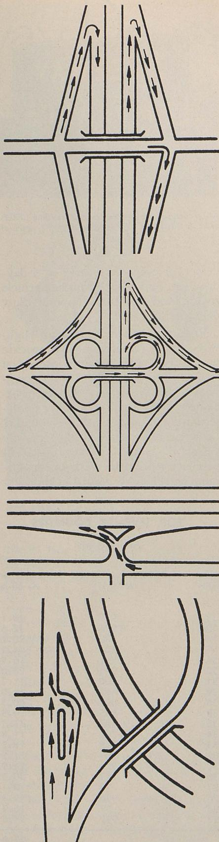
Typical wrong-way movements at various types of interchanges are (top to bottom): diamond; cloverleaf; buttonhook; and cul-de-sac (design of channelization variable).
