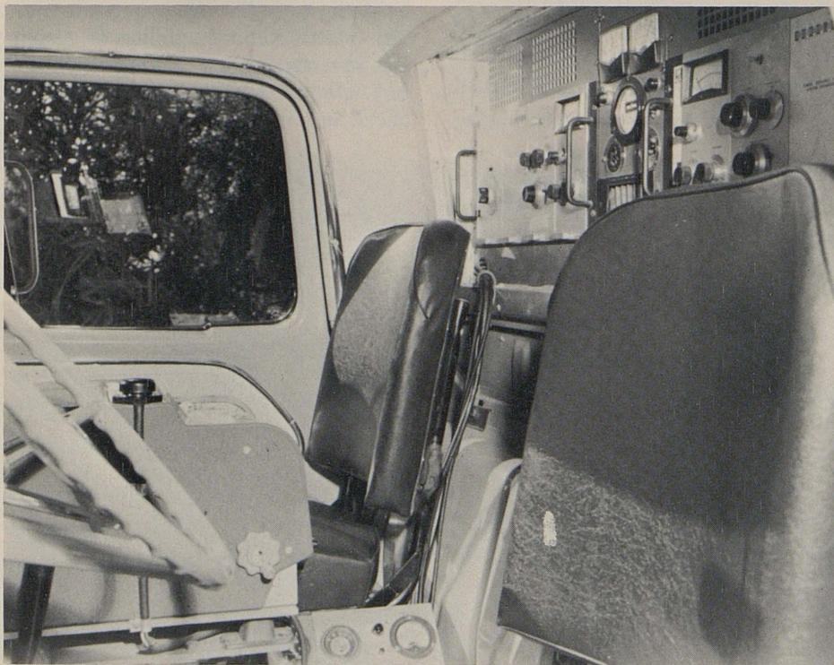
FIGURE 5—The recording unit and electronic equipment may be regulated by the driver or his assistant.
