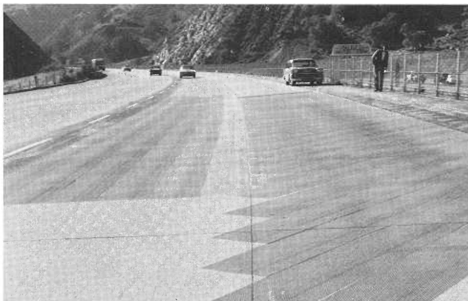
Below: Overall view of test area on Route 5 in Kern County, showing diagonal and longitudinal scoring of a portland cement concrete pavement for improving its skid resistance.
