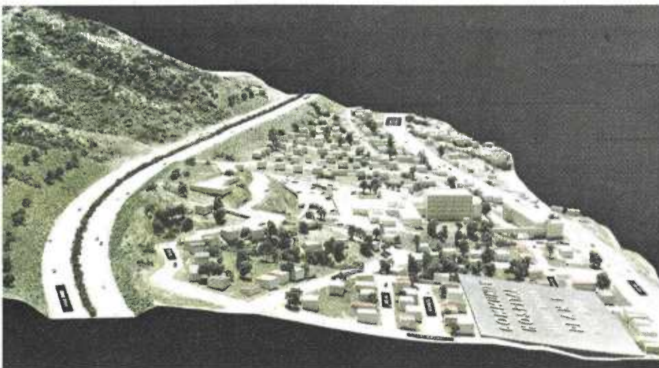
Above and left: Models of this type are constructed so that geometrics of traffic service, physical relationship to adjacent property, highway safety and aesthetic impact may be studied during design of a project.
