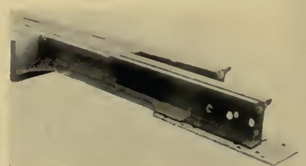
Broken switch casting after repairs have been made
