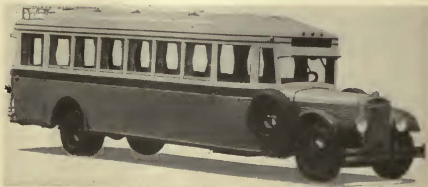
The Parlor body on the 233-in. wheelbase chassis will accommodate 29 passengers, while the 265-in. wheelbase type can carry a parlor body for 33 passengers
