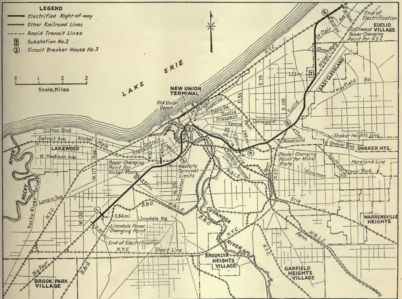
The electrified zone extends from Collinwood on the east to Linndale on the southwest, a distance of 17 miles. The present routes of the New York Central, Nickel Plate, Big Four, Baltimore & Ohio, Erie and Wheeling & Lake Erie and how these roads will or will be able to tie into the new right-of-way are shown
