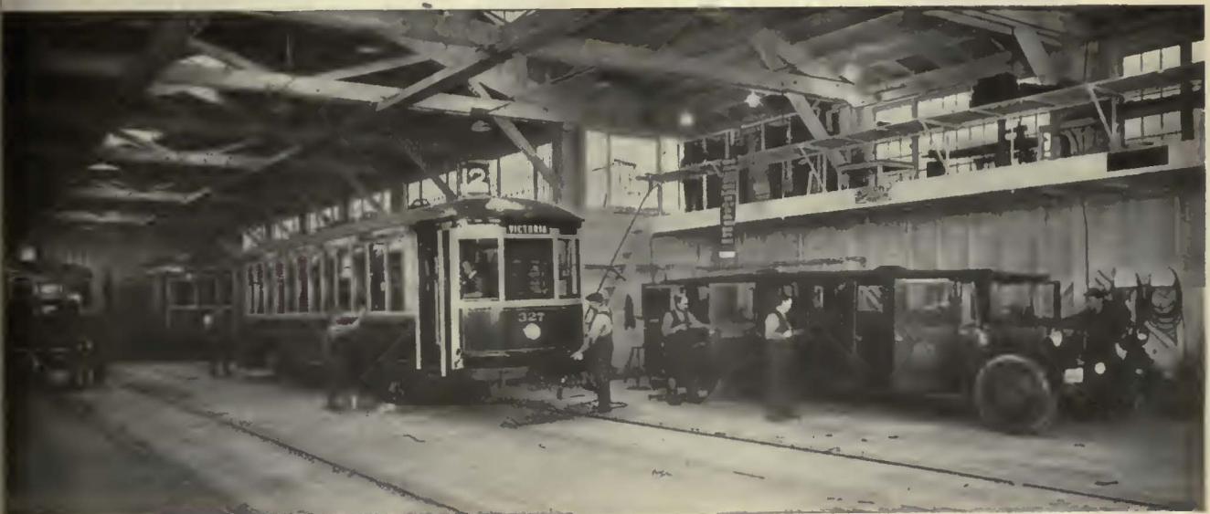
Interior of paint shop of the British Columbia Electric Railway. Both cars and buses are refinished. The gallery at the right is used for sign repairs
