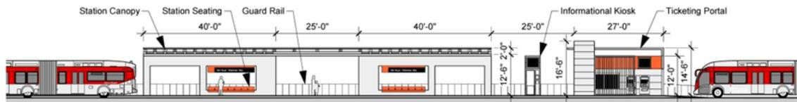
**03** MEDIAN BRT PLATFORM ELEVATION
