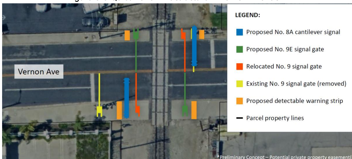
Figure 3-3 Quiet Zone Infrastructure – Vernon Avenue
