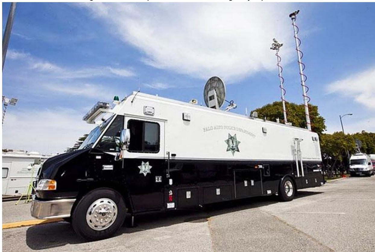
Figure 3-2 Example of a Mobile Emergency Operations Center
