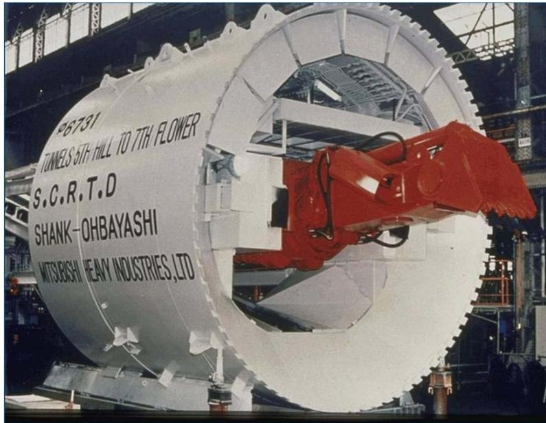
Open-face shield tunneling has the advantage that when an obstruction, such as a tie-back is encountered, it can be more easily removed via openings in the shield as illustrated in Figure 2.2-12. The tunnel face is accessible and the tie-back can be removed in pieces manually by torch cutting or metal cut-off saw. It is a time-consuming effort that requires grouting where unstable soils are present.
