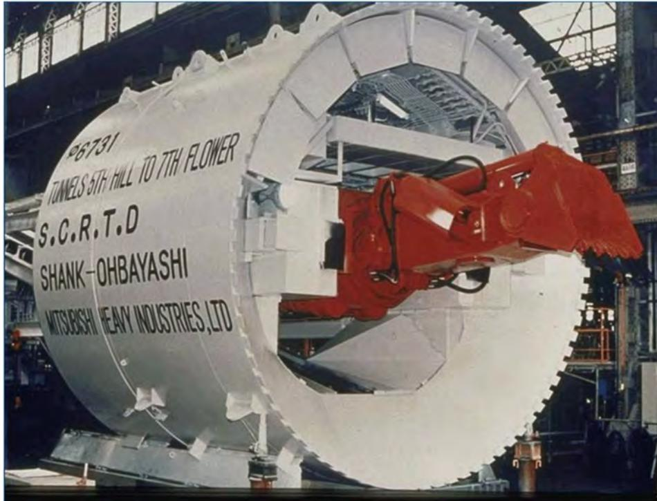
A characteristic of a digger shield is that, when an obstruction such as a tieback is encountered during tunneling, the tunnel face is accessible and the tieback can be removed in pieces manually by torch cutting or metal cut-off saw. Special powered equipment operated remotely by miners would likely be used to assist in tieback removal to some extent. Regardless of possible mechanized assistance, manual labor would be required and job-specific safety hazards would exist for tieback removal.
