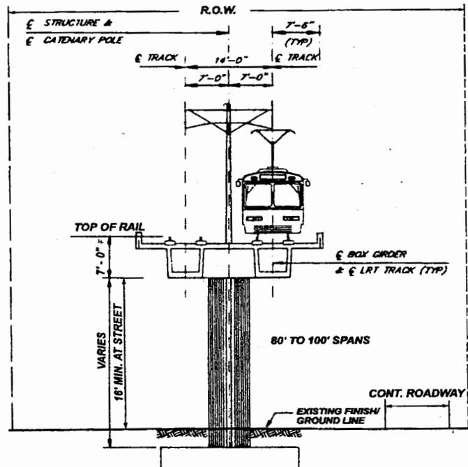
NOTE: CATENARY AND PANTOGRAPH SYSTEM APPLIES TO ALTERNATIVES 6 AND 11.
