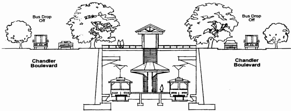
Open Air Underground Station (Center or Side Platform)
