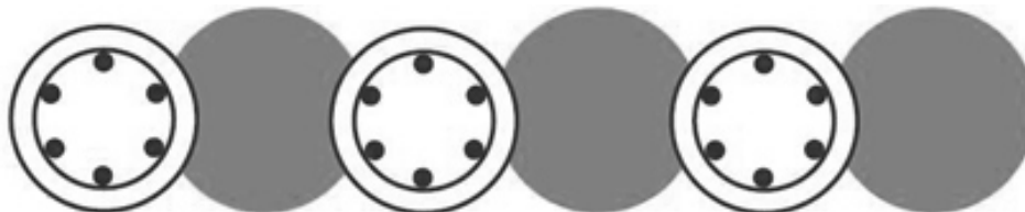
FIGURE 4-11. SECANT PILES AND REINFORCEMENT ARRANGEMENT
