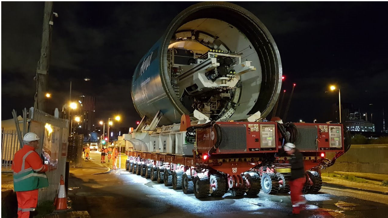
FIGURE 4-4. TUNNEL BORING MACHINE DELIVERY
