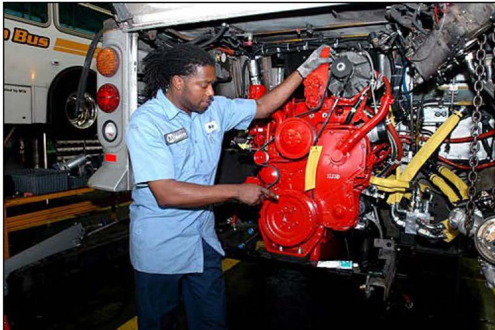
Explaining what work remains, Mustafa Bey, mechanic "B," stands beside a newly-installed Cummins 8.9 ISL-G engine. Photos by Ned Racine
