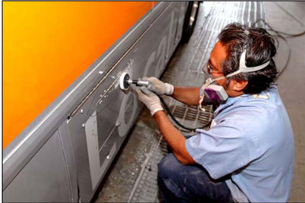
David Garcia, a body repairer "A," removes corrosion from a New Flyer Hi-Floor 5000 series bus. The bus has already been steam cleaned and had its decals removed.
