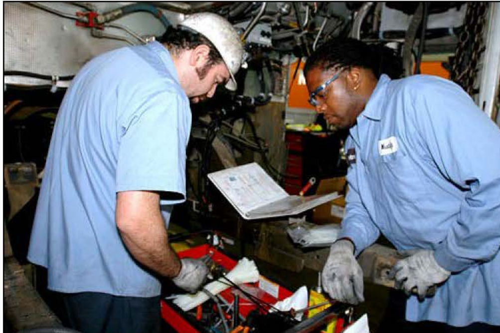
Sergio Renteria, mechanic "A" and Mustafa Bey, mechanic "B" replace connectors for transmission diagnosis as part of the Re-Power process.
