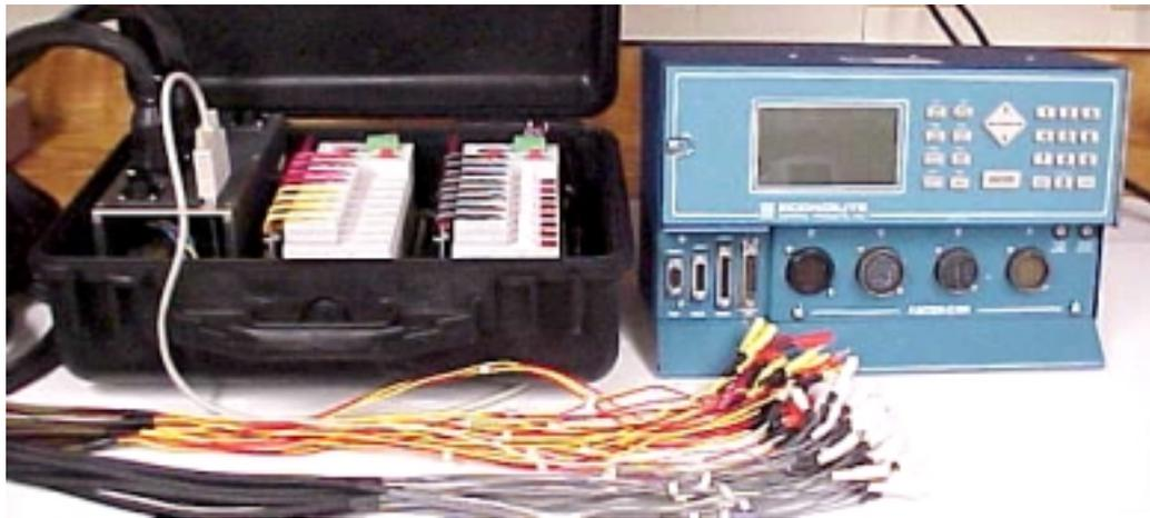
a) CID and Signal Controller (No Feasible Connection)
