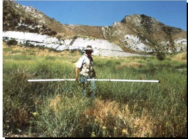
***Geonics EM-31 Terrain Conductivity Meter***
