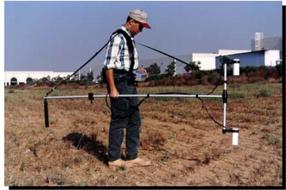
**Geometrics G858 Cesium Magnetic Gradiometer**
