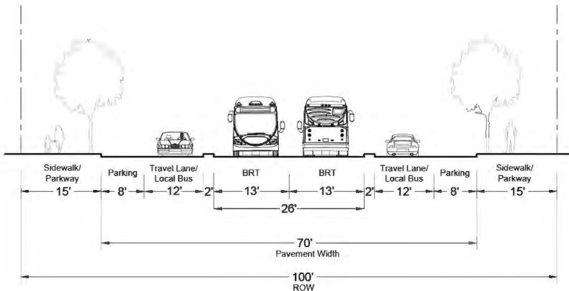
Figure 27 depicts a rendering of two center-running dedicated BRT lanes south of Gage Avenue. This configuration can be achieved by converting one travel lane in each direction to a bus only lane.
