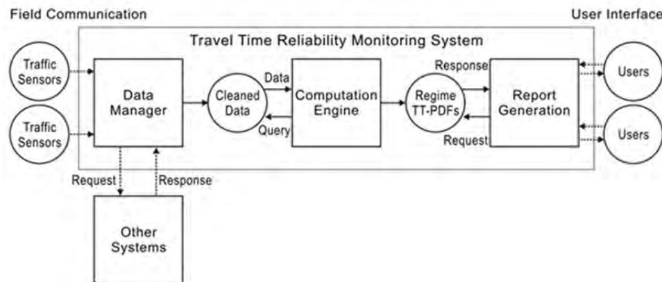
Figure 3-1: The Travel Time Reliability Monitoring System
