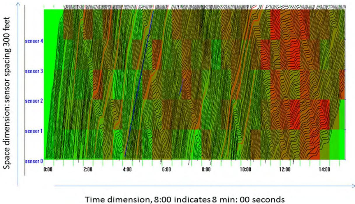
**Figure 5-14: Space-time vehicle trajectory and aggregated density representation with a sampling rate of 30 seconds and 300 feet, color coded from green to red representing the aggregated density from low to high**
