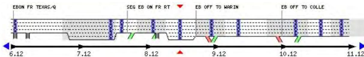
**Figure 5-1: Typical Sensor Spacing on a Freeway**
