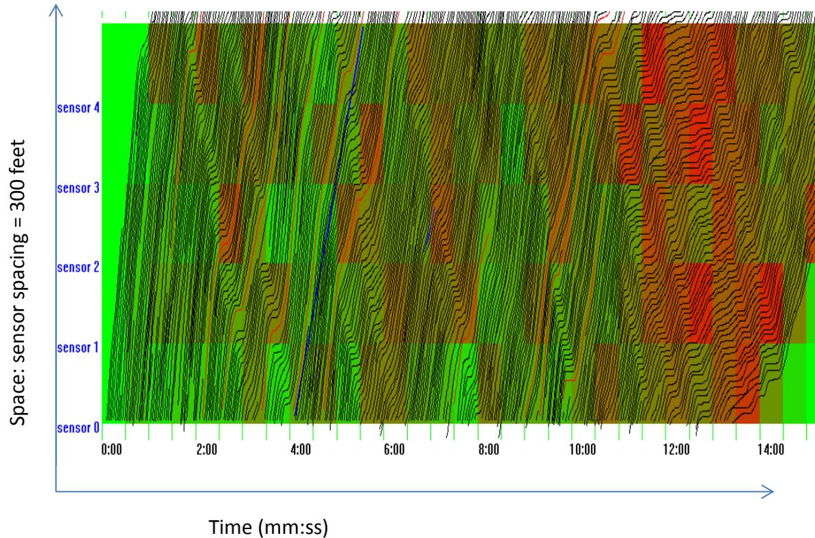
**Figure 5-3: Vehicle trajectories in space and time**
