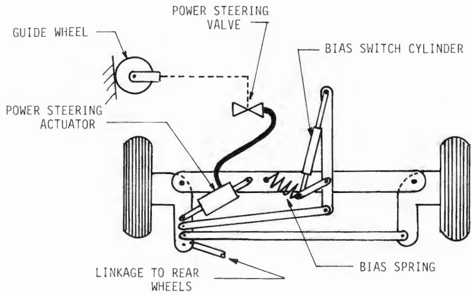
(a) SIMPLIFIED DIAGRAM OF STEERING AND SWITCH SYSTEM
