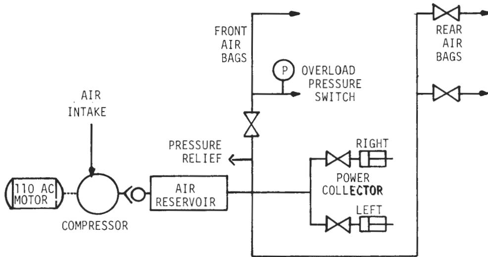
FIGURE 3.12 : SIMPLIFIED PNEUMATIC SYSTEM SCHEMATIC
