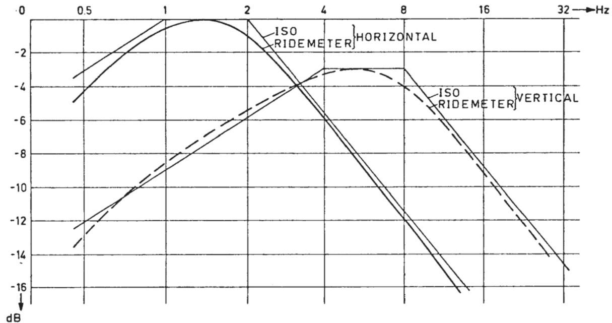
FIGURE 4.27: COMFORTMETER FILTER CHARACTERISTICS
