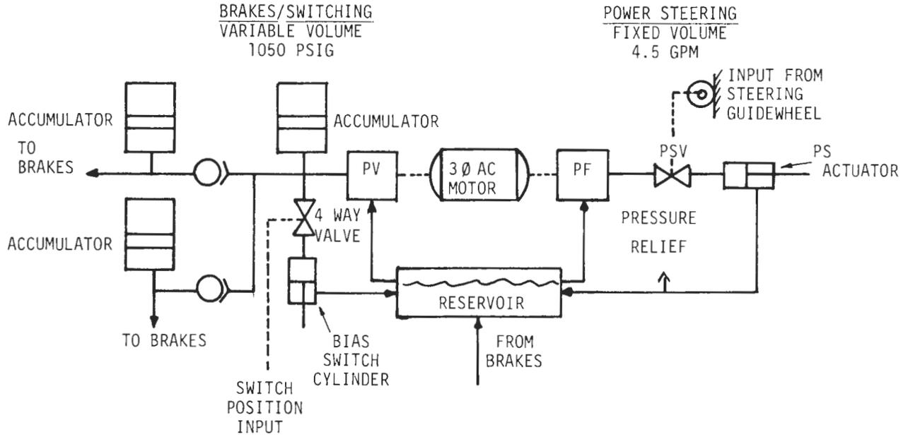
FIGURE 3.11 : SIMPLIFIED HYDRAULIC SYSTEM SCHEMATIC
