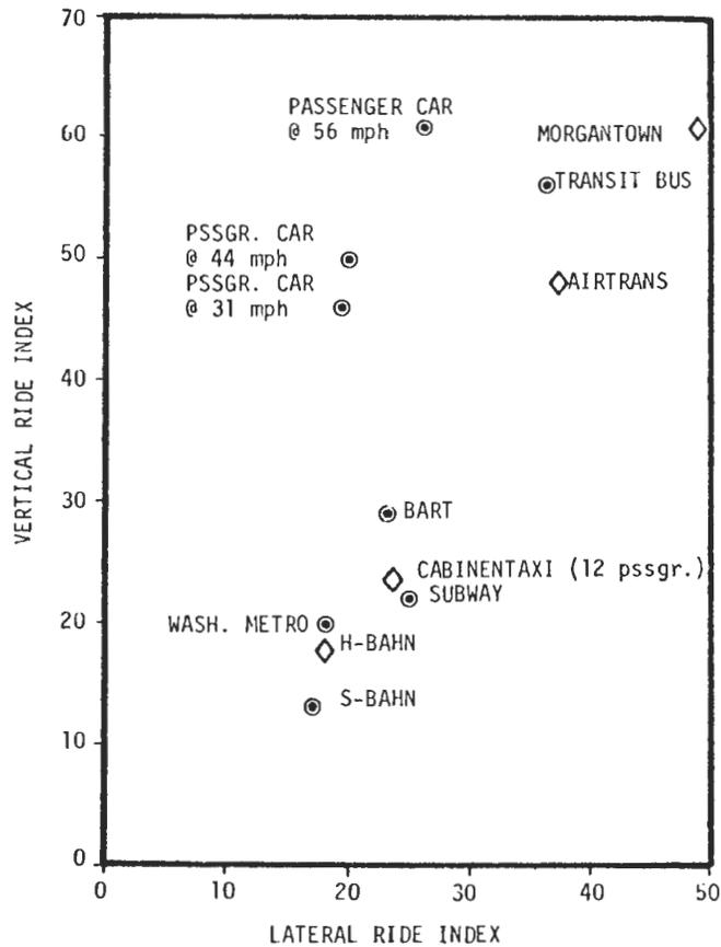
FIGURE 4.33: AVERAGE LATERAL AND VERTICAL RIDE INDEX VALUES FROM ALL MEASUREMENTS
