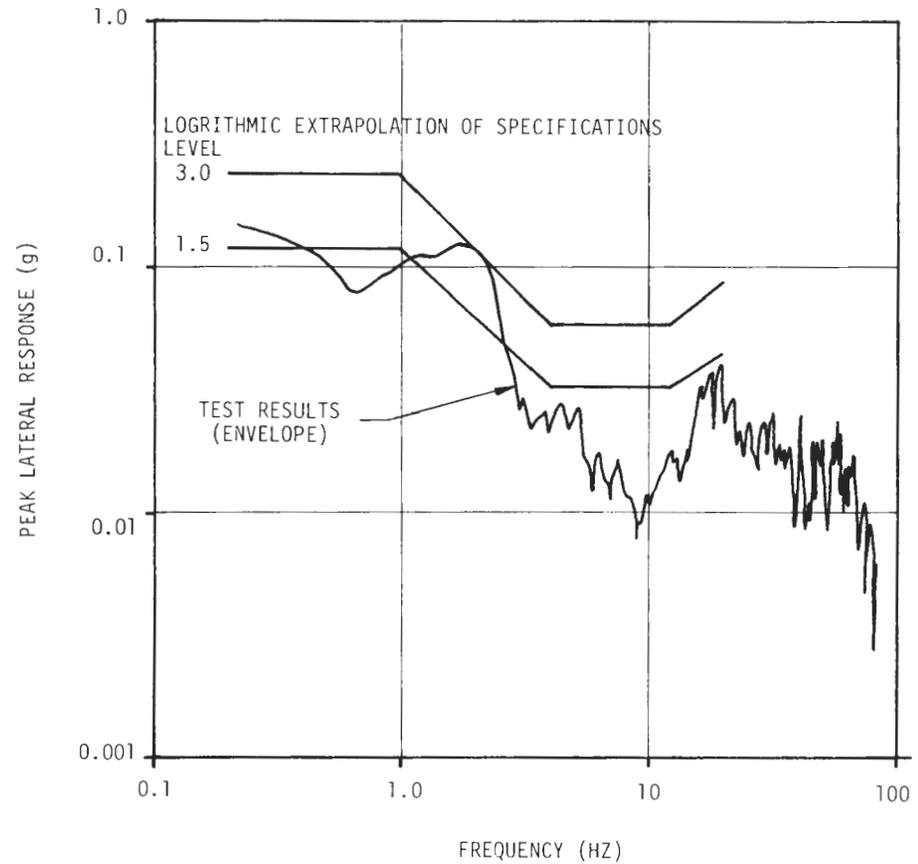
FIGURE 4.26 : MAXIMUM ENVELOPE OF REPRESENTATIVE FOURIER TRANSFER FUNCTIONS FOR LATERAL RESPONSE, BOEING RIDE COMFORT TESTS
