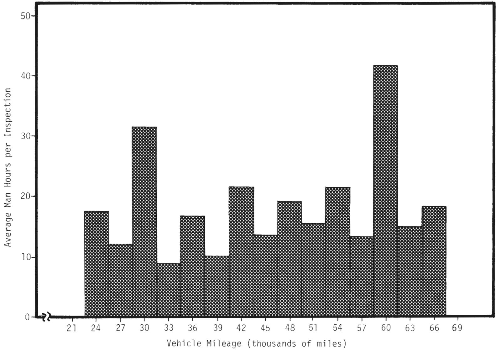
FIGURE 4.14: SCHEDULED VEHICLE MAINTENANCE - AVERAGE MAN HOURS PER 3,000-MILE INSPECTION
