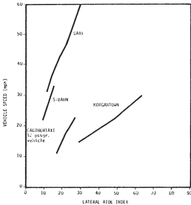
FIGURE 4.31: COMPARISON OF LATERAL RIDE QUALITY FOR DIFFERENT TRANSIT SYSTEMS
