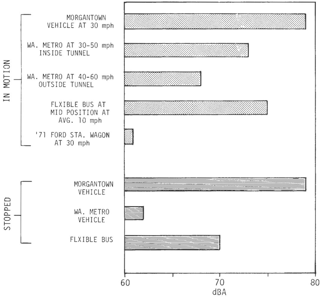
FIGURE 4.39: COMPARISON OF INTERIOR NOISE (dBA) FOR DIFFERENT TRANSIT VEHICLES
