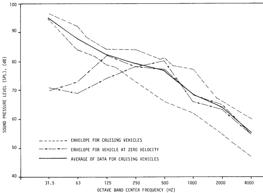
FIGURE 4.35 : INTERIOR NOISE IN RANDOMLY SELECTED VEHICLES AT VARIOUS SPEEDS AND CONDITIONS
