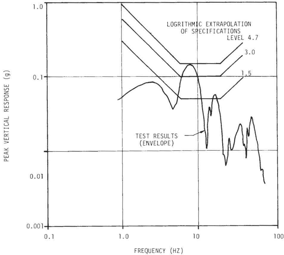
FIGURE 4.25 : MAXIMUM ENVELOPE OF REPRESENTATIVE FOURIER TRANSFER FUNCTIONS FOR VERTICAL RESPONSE, BOEING RIDE COMFORT TESTS
