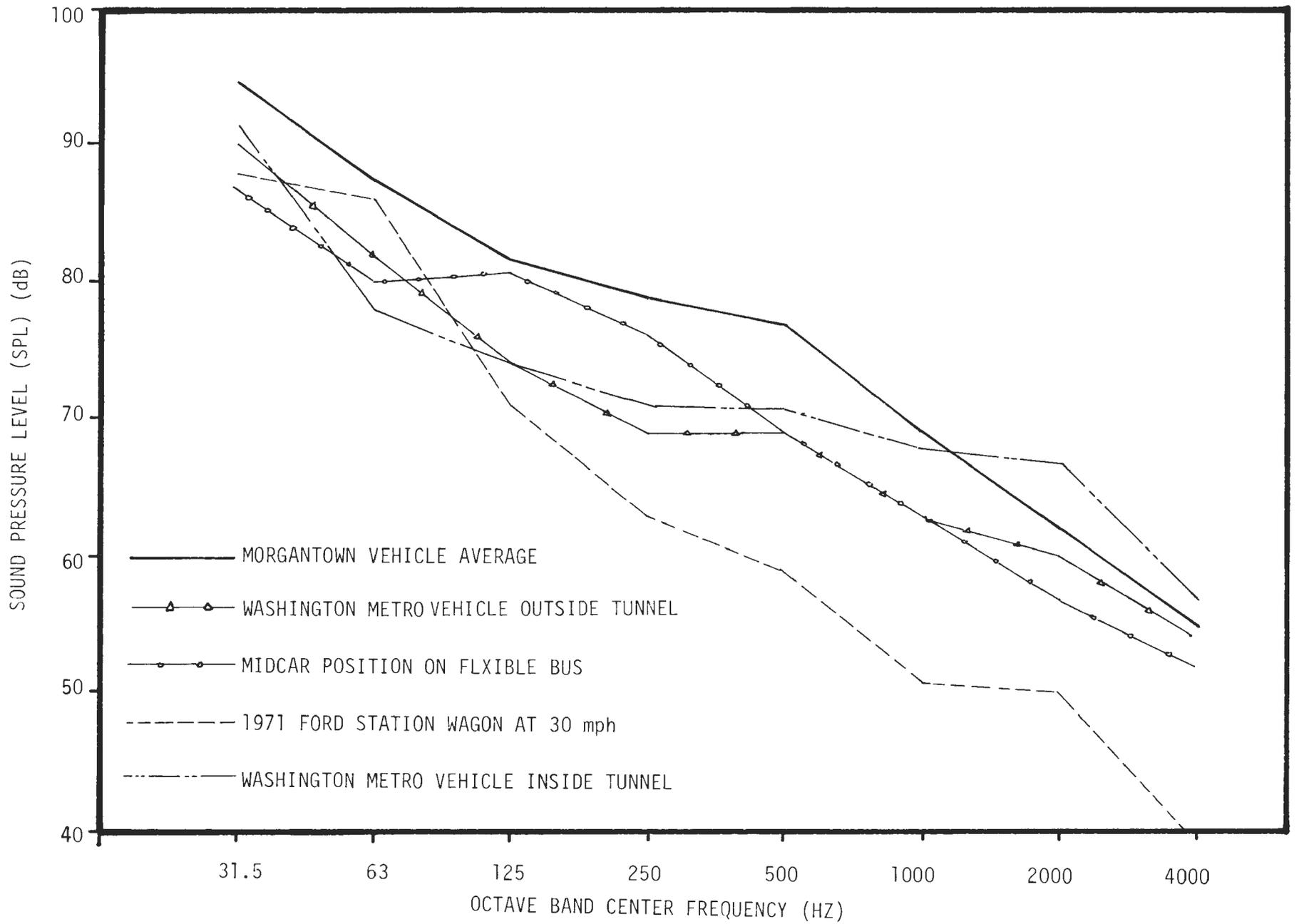
FIGURE 4.38 : COMPARISON OF INTERIOR NOISE FOR DIFFERENT TRANSIT VEHICLES
