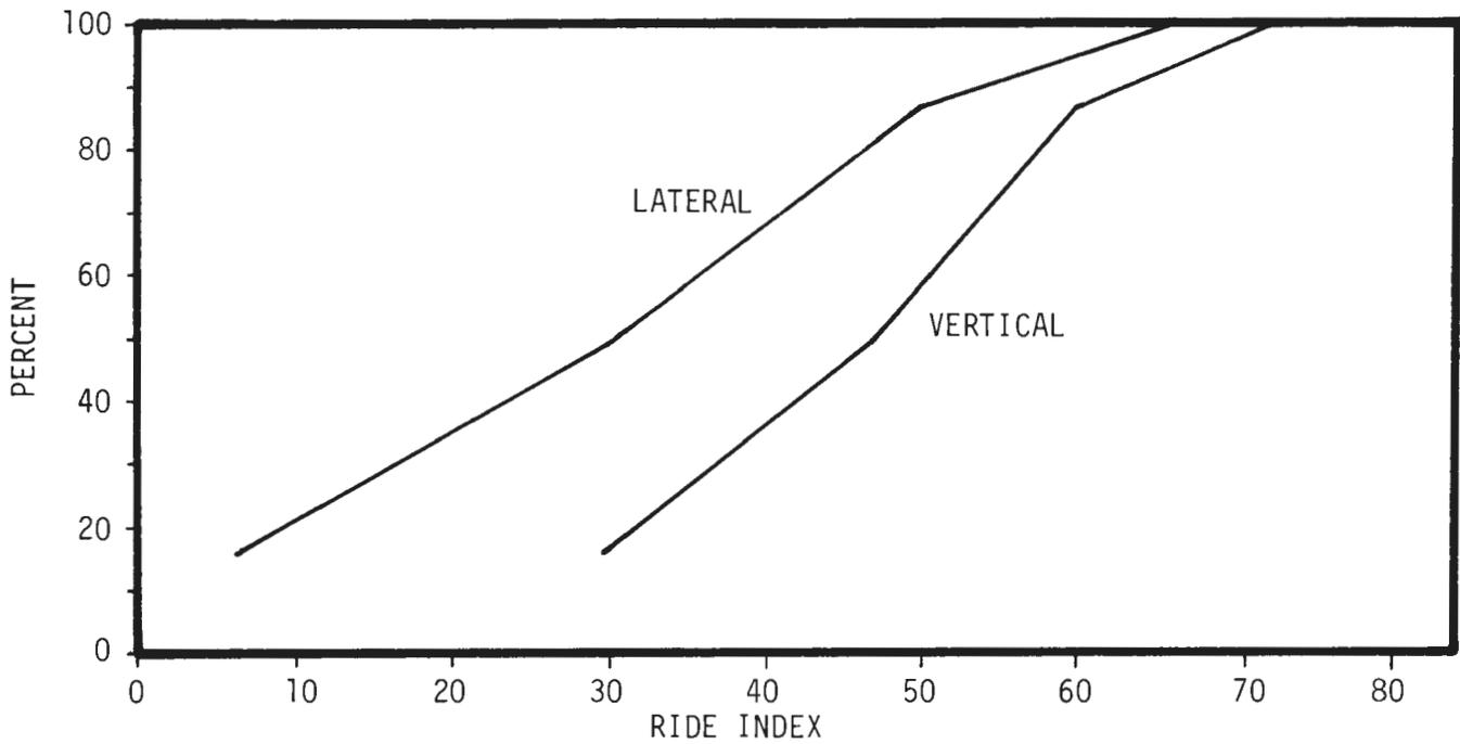
FIGURE 4.29 : PERCENTAGE OF TRIP TIME DURING WHICH VERTICAL OR LATERAL RIDE INDEX IS NOT EXCEEDED (ENGINEERING - WALNUT)
