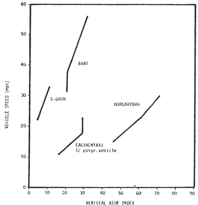
FIGURE 4.32: COMPARISON OF VERTICAL RIDE QUALITY FOR DIFFERENT TRANSIT SYSTEMS
