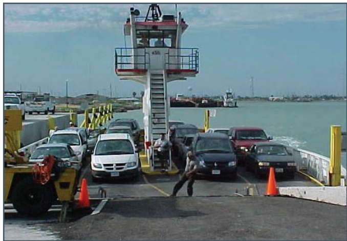
Figure 2.20 Temporary vehicular ferry
