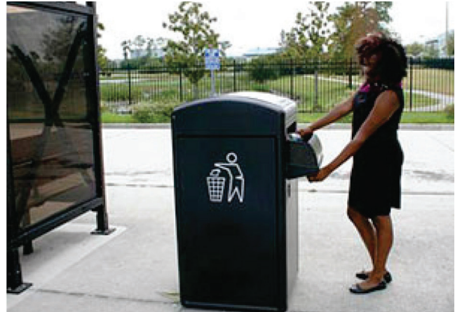
FIGURE 7 Solar trash compactors in Pinellas County, Florida, reduce the frequency of required trash removal.
