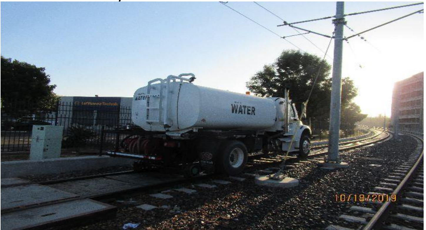
EUCALYPTUS STREET - HCC hi-rail water truck at grade crossing STA 182+25 SB #3 track.
