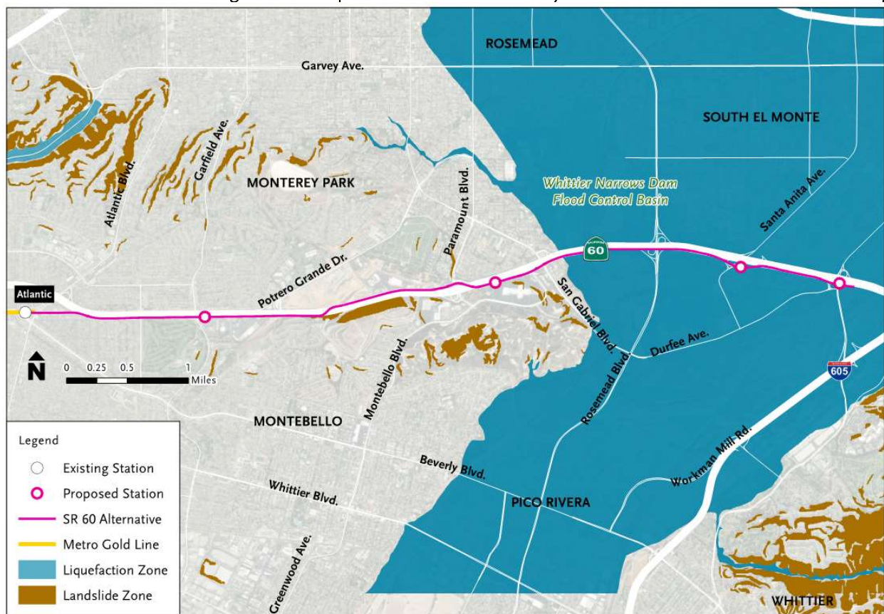
Figure 4-1. Liquefaction and Seismically-Induced Landslide Hazard Zone Map
