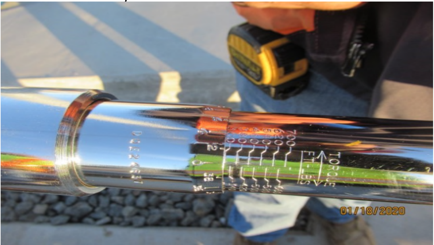
Florence/Brea – WSCC calibration wrench set for 300 FT.LBS prior to verifying DF fastener bolts on LA Brea bridge
