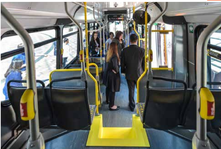
Example of push buttons located at lower heights and locations on a new Metro El Dorado CNG bus (2018)
