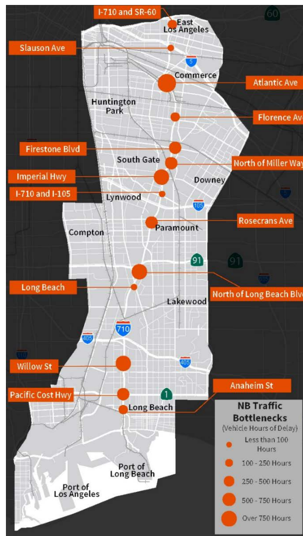
Figure 3-68. Northbound Bottlenecks Along I-710
