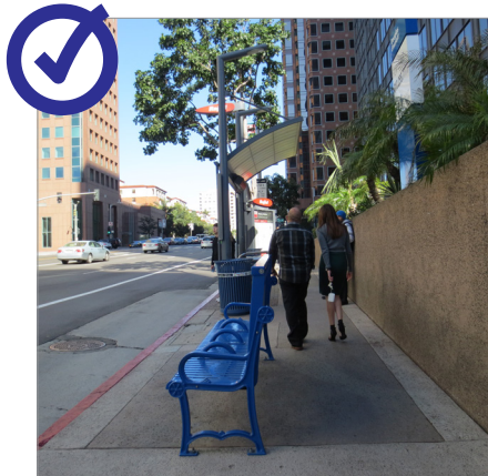
There are two distinct zones: the Sidewalk Stop and a throughway for passing pedestrians (Westwood, LA)
