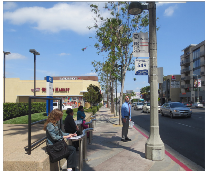
The narrow Sidewalk Stop efficiently provides customers with seating, lean bars, shade trees, and Sidewalk Stop identification and transit information integrated on a light pole (Sepulveda Blvd, Sherman Oaks)
