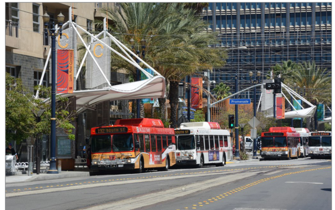
Direct Connections Ideally, transfers are direct and do not require crossing any streets, driveways or other points of conflict with vehicles (Long Beach Transit Mall, Long Beach)
