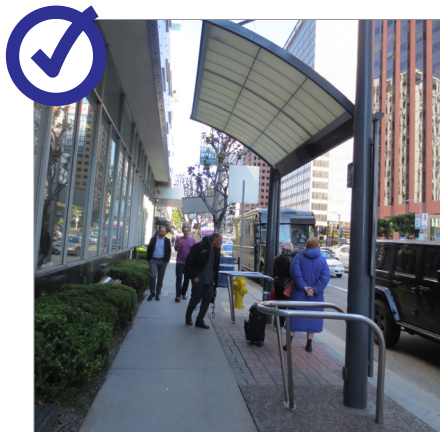
Where space for shelters and seating is limited, smaller shelters and lean bars are good alternatives (Westwood, LA)
