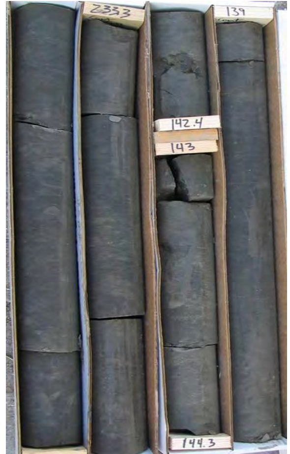
Figure 4-4. Fernando Formation. Core from boring R-09-Z4B4 at a depth of 139 to 144 feet and 233 to 238 feet, showing consistent nature of unbedded siltstone/mudstone.
