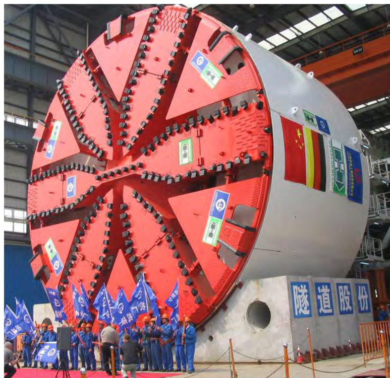
Figure 2: TBM Used to Mine the Shanghai Yangtze River Tunnel (Source: Herrenknecht, 2009)
