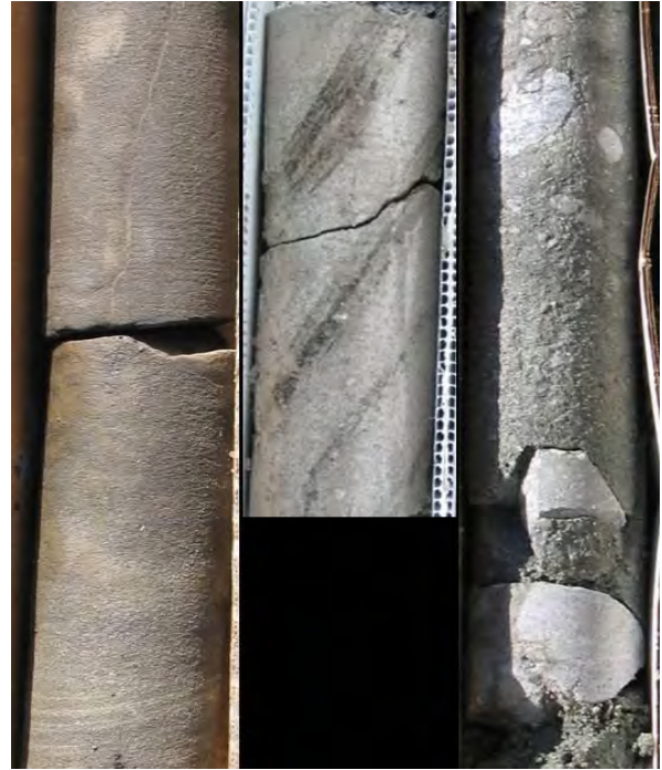
Figure 4-6. Topanga Formation. Core on right is conglomerate with sandstone matrix from boring R-09-Z3B6 at a depth of 223 to 226 feet; core in middle is sandstone with siltstone laminations from boring R-09-Z3B7 at a depth of 253 feet; core on left is siltstone/mudstone from boring R-09-Z3B8 at 258 feet.
