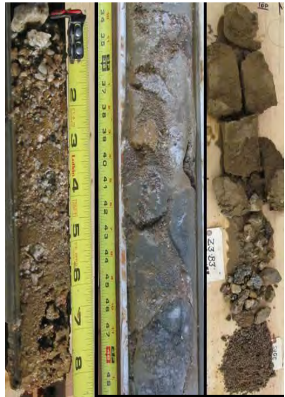
Figure 4-3. Alluvium. The three cores show a variety of sandy and gravelly alluvium from boring R-09-Z3B3. The core on the left is coarse sand and fine gravel from depths of 130 to 133 feet; the core in the middle is coarse gravel from 154 to 159 feet; the core on the right is sand and gravel from 30 to 31 feet.
