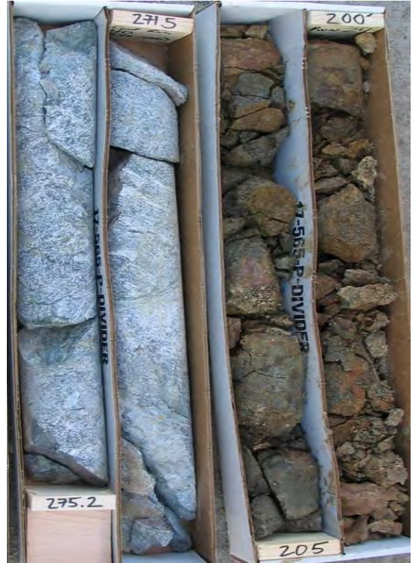
Figure 4-7. Basement Rocks. Igneous and metamorphic rocks from boring R-09-Z3B4. The two cores on right are weathered rocks from a depth of 200 to 205 feet. The two cores on left are fresh rock from 271 to 275 feet.
