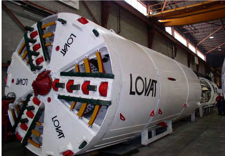
Figure 1: Pressurized-Face TBM Equipped with Cutterhead for Rock and Soil
