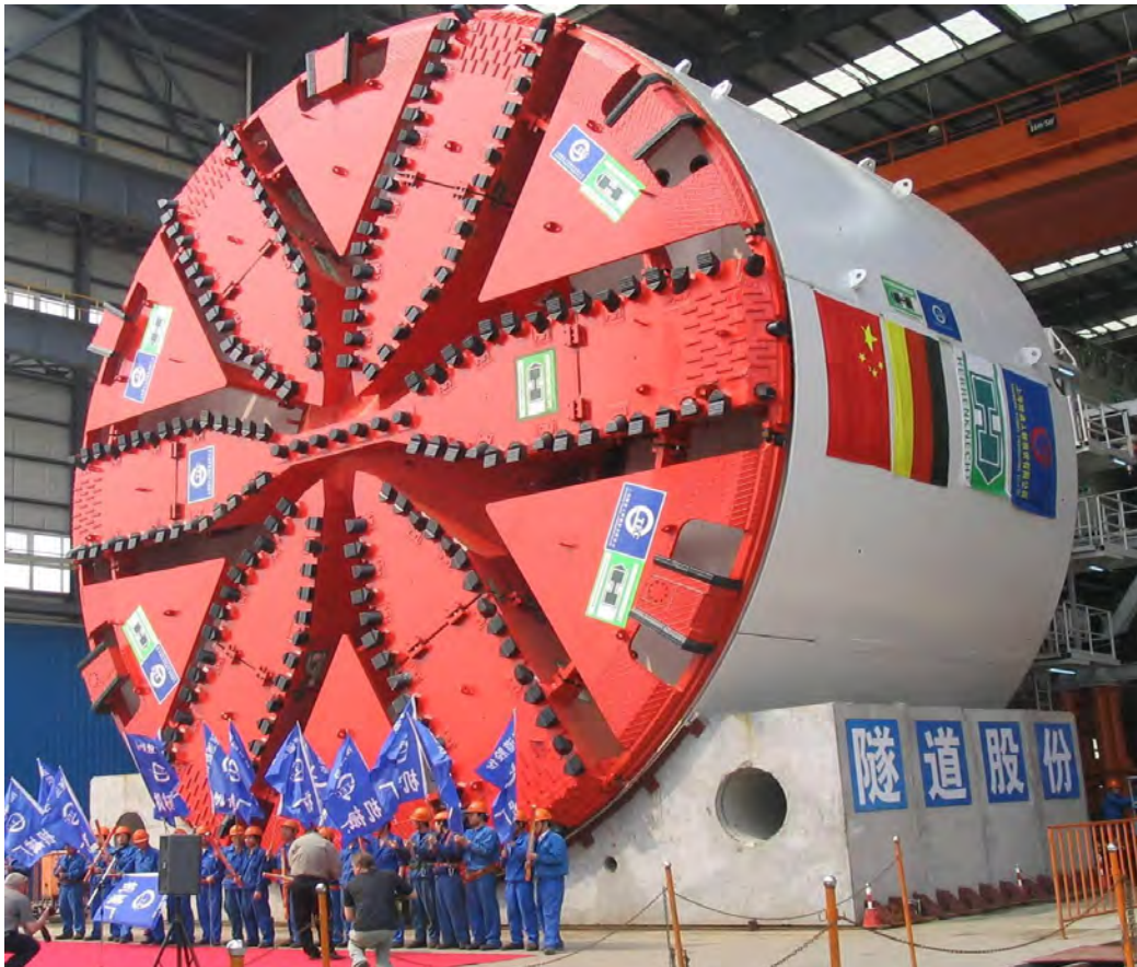
Figure 12-9. Largest TBM in the world to date, for the Shanghai Yangtze River Tunnel Project (Herrenknecht, 2009).
