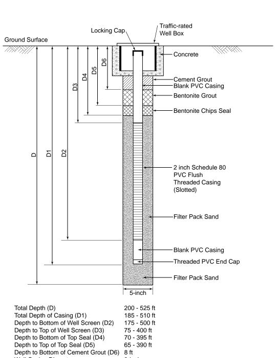
Well Casing Diameter 2-inch Well Screen Slot Size 0.020-inch Filter Pack Sand Type Monterey No. 3 Medium Chips Bentonite Seal Type
