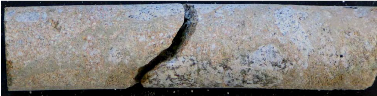
Failed core from 06-3, 106.5 ft depth
