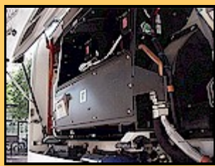
MTA Equipment Engineering Mechanic John Mirabal inspects Thermal King air conditioning system on a new compressed natural gas bus manufactured by North American Bus Industries (NABI). The electronically controlled air conditioning system can drop the temperature inside the bus from 80 degrees to 68 to 72 degrees in approximately six minutes.
