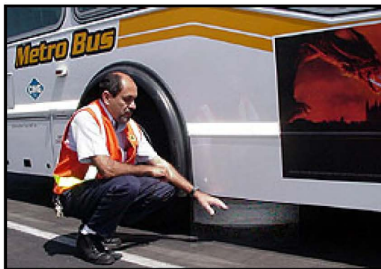
Joe Quintero, Division 9 equipment maintenance supervisor, points out the Dangerzone Deflector that can push a fallen pedestrian out of harm's way. Below, stills from a Dangerzone Deflector video show the deflector pushing aside a fallen pedestrian.
