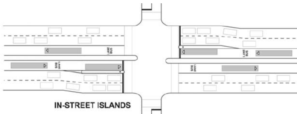
Figure 7.3 Treatment for Median Bus/BRT/Light Rail Stops
