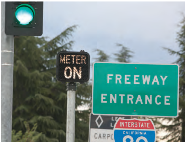
Freeway ramp meter indicator.
