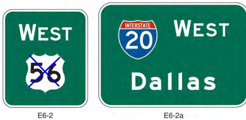
Figure 2E-2. Pull-Through Signs
