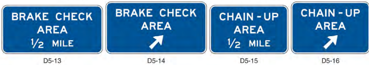
Figure 2I-6. Brake Check Area and Chain-Up Area Signs
