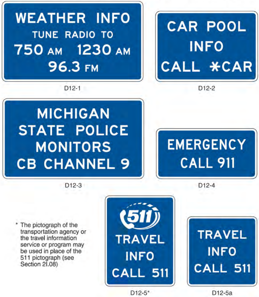
Figure 2I-8. Radio, Telephone, and Carpool Information Signs
