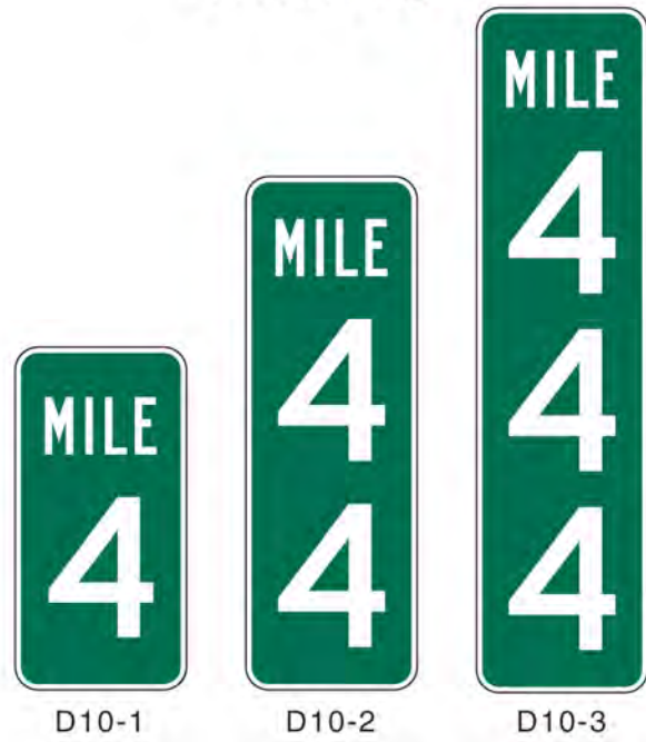
Figure 2H-2. Reference Location Signs
