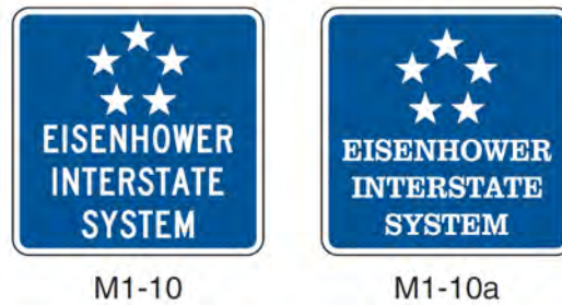
Figure 2E-18. Eisenhower Interstate System Signs
