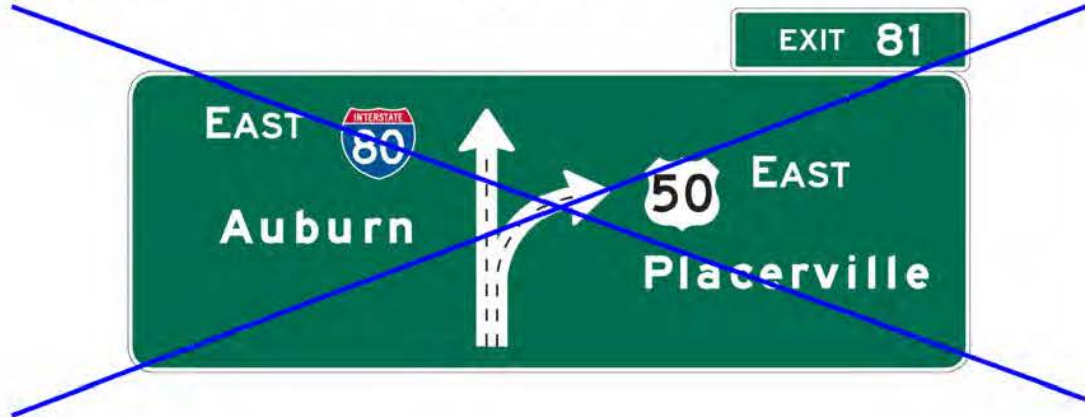
Figure 2E-7. Diagrammatic Guide Sign for a Multi-Lane Exit with an Option Lane
