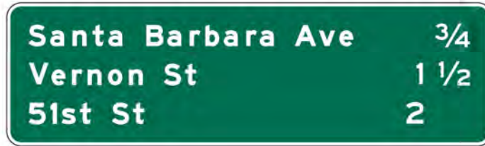
Figure 2E-31. Interchange Sequence Sign
