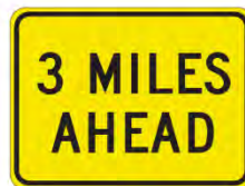
Figure 2C-12 (CA). Supplemental Warning Plaques
