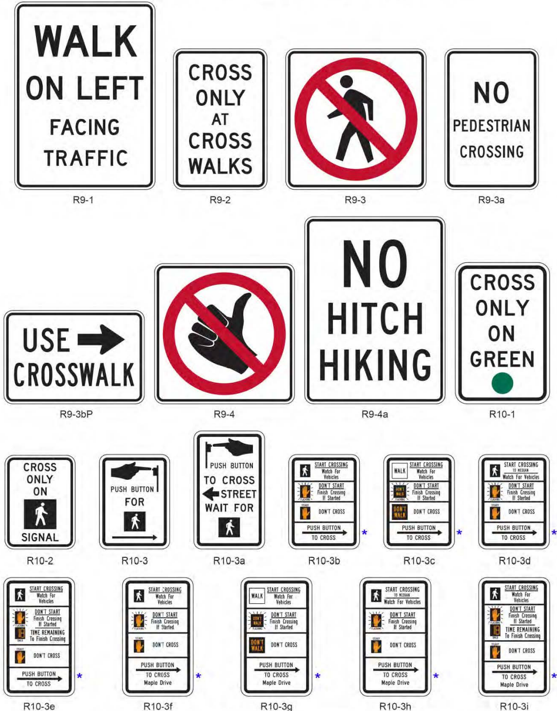
Figure 2B-26. Pedestrian Signs and Plaques (Sheet 1 of 2)
