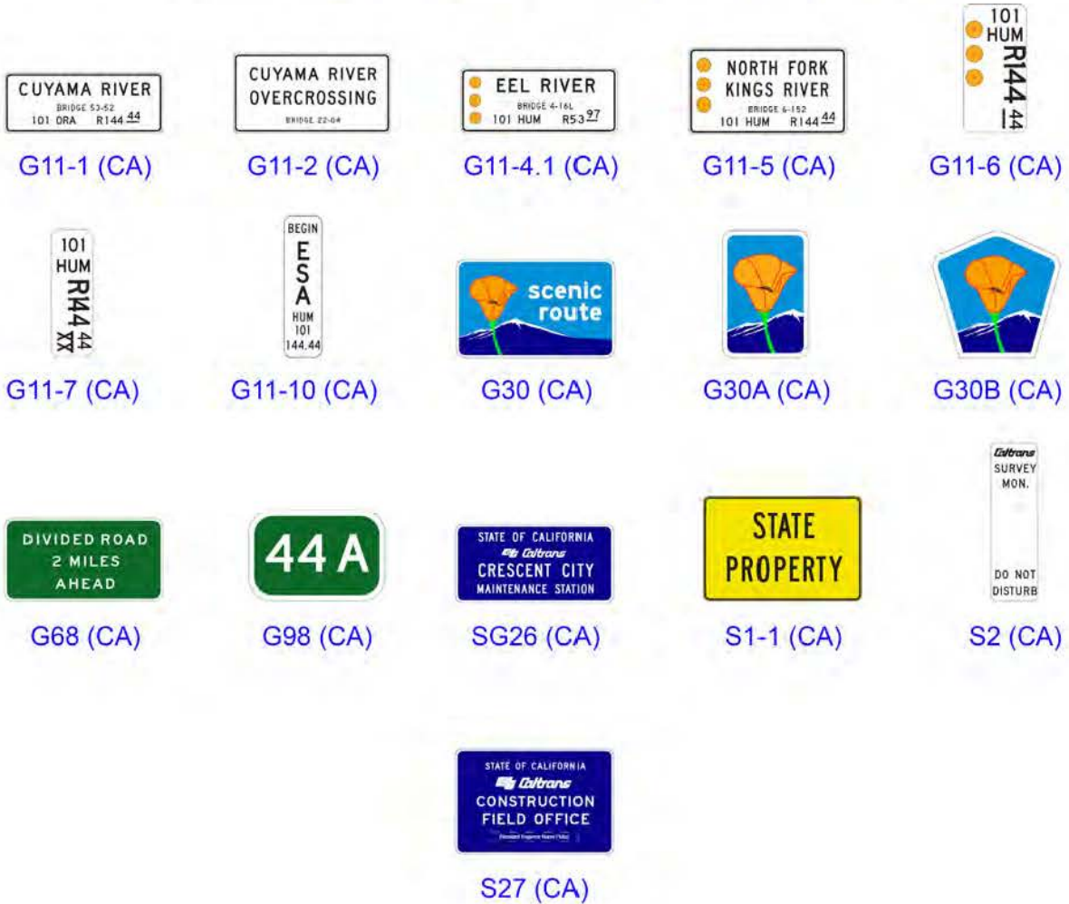
Figure 2D-101 (CA). California Miscellaneous Guide Signs
