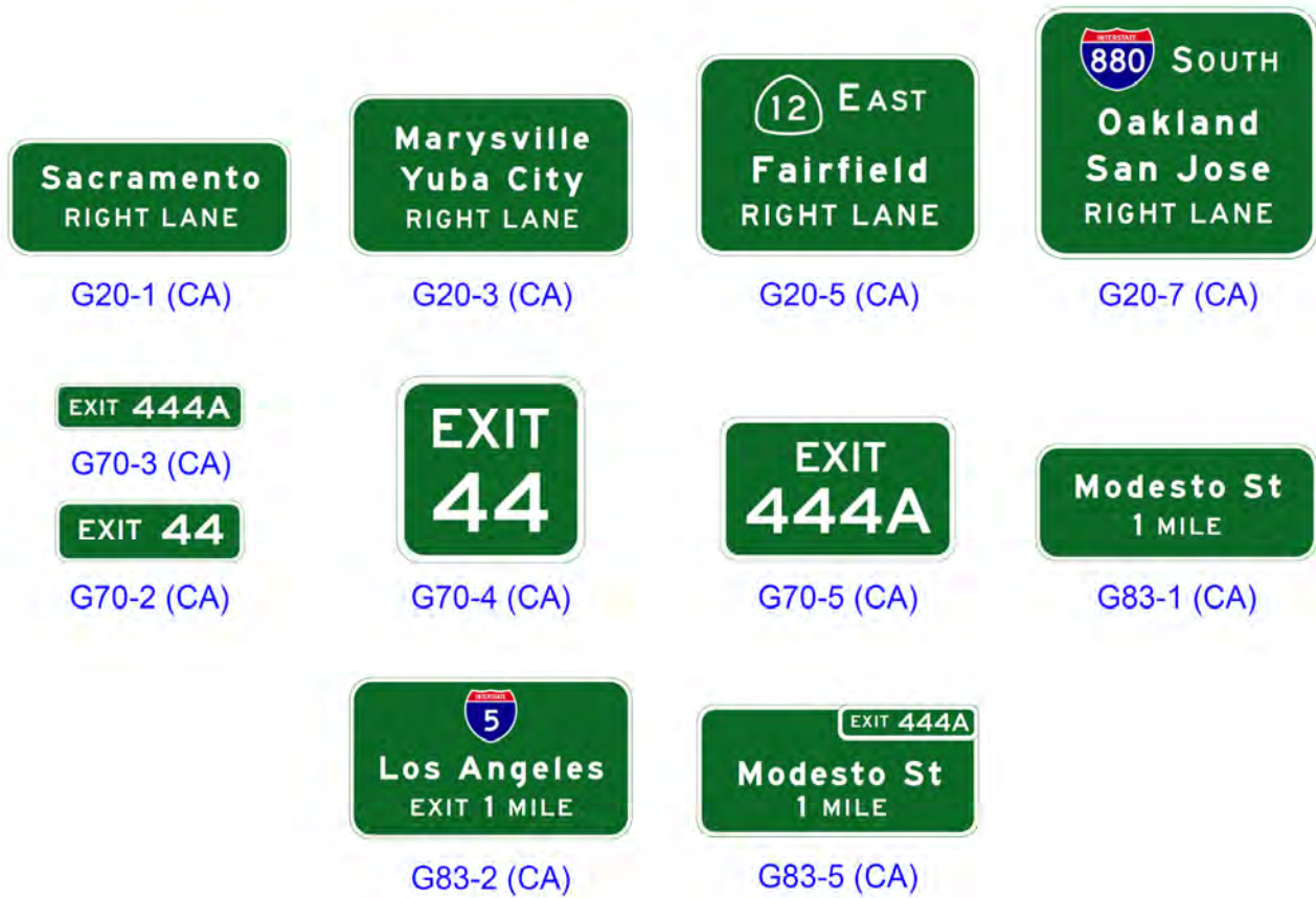
Figure 2E-22 (CA). Examples of Interchange Advance Guide Signs, Exit Number Plaques, and LEFT Plaque
