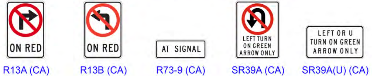
Figure 2B-27 (CA). Traffic Signal Signs and Plaques
