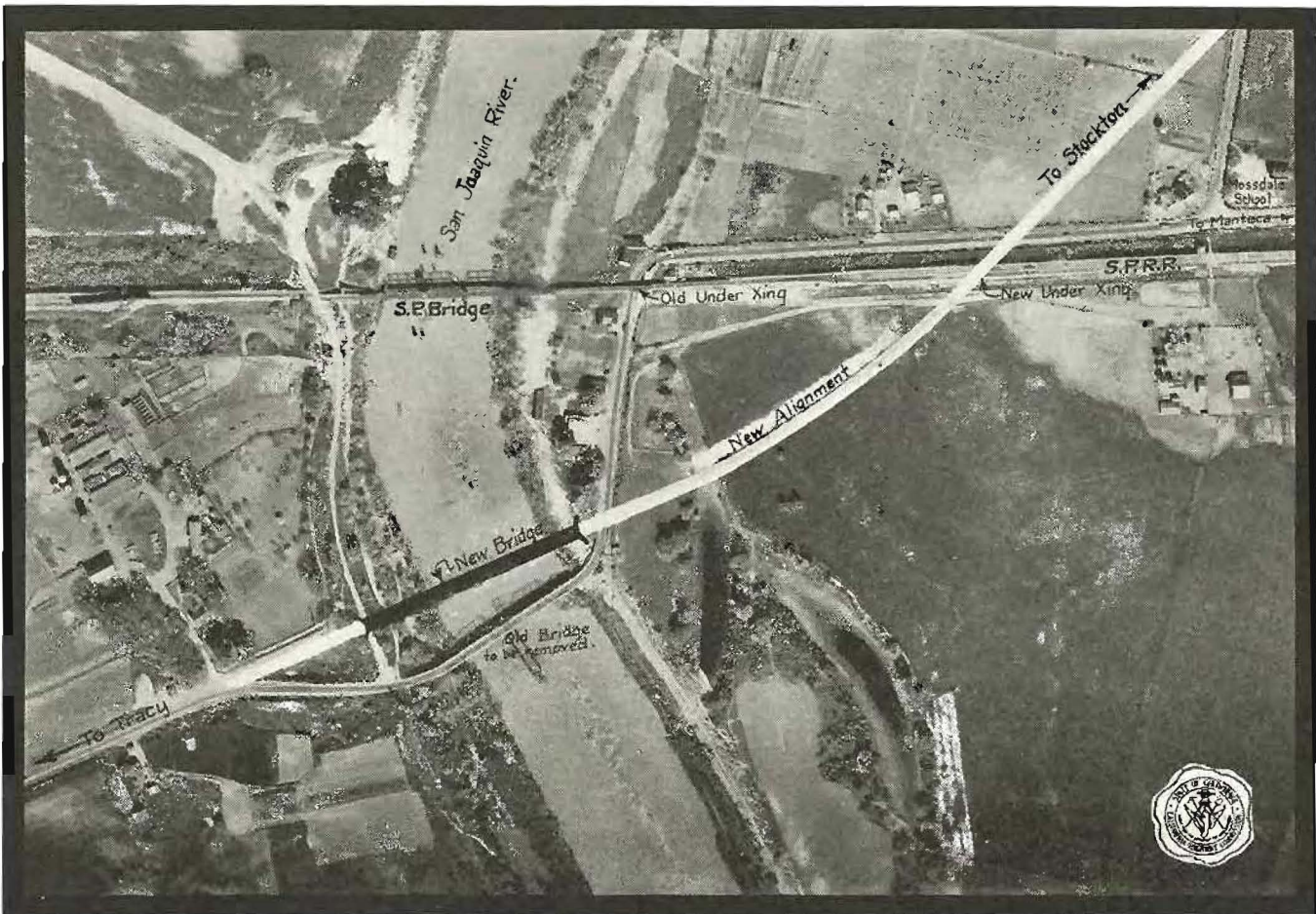
MOSSDALE FROM THE AIR—A contract has been awarded for the new bridge at the location indicated in the airplane view secured through the cooperation of the United State Air Service. Rights of way also have been deeded the state by the county for the realignment of the highway, substituting two easy curves for six almost at right angles.
