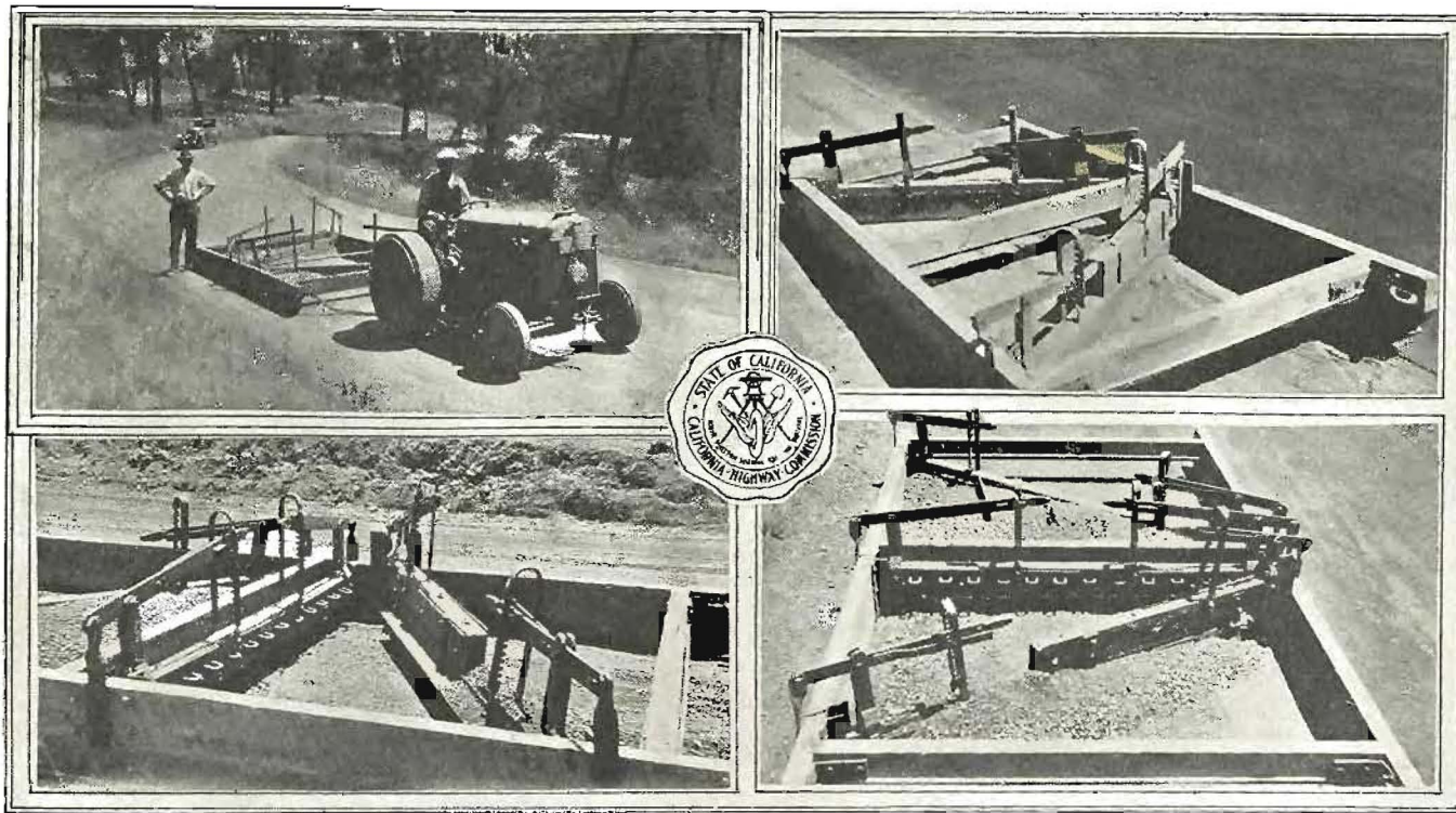
DIVISION VI BUILDS DRAG—Views show equipment development by maintenance forces of Division VI for dragging of shoulders and earth and rock surfaced highways.
