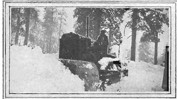
Snow removal by push plow on rock-surfaced Fredonia summit between Westwood and Susanville, Lassen County.
