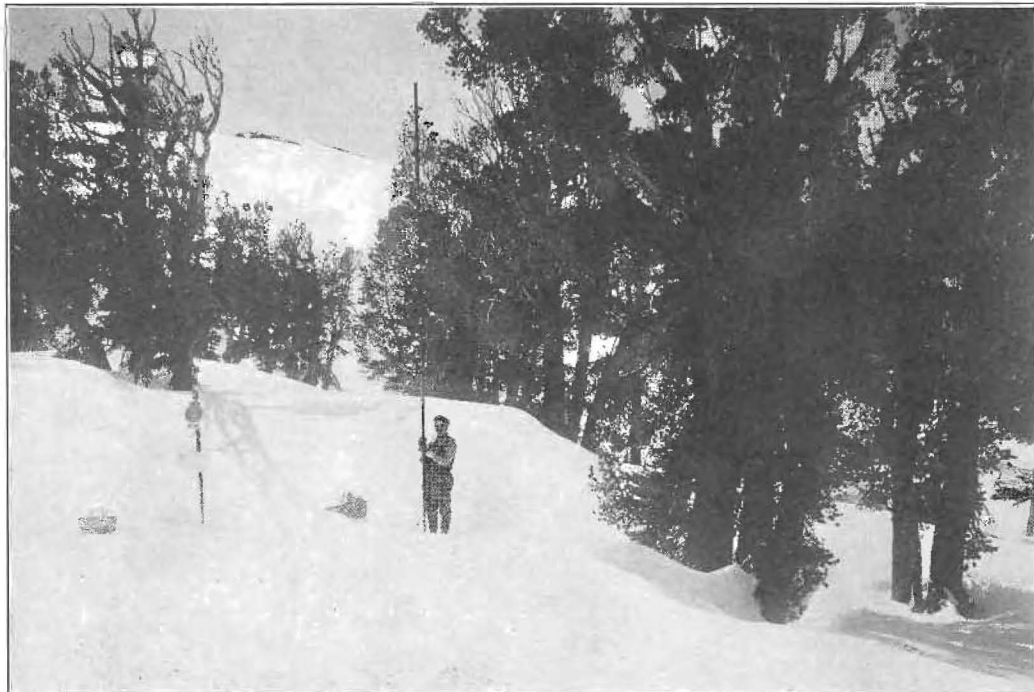
Sampling the snow at Mt. Rose. The snow is as deep as the sampler is long.
