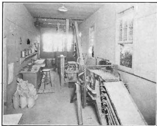
Coarse aggregate department, showing abrasion, crushing and screening equipment.
