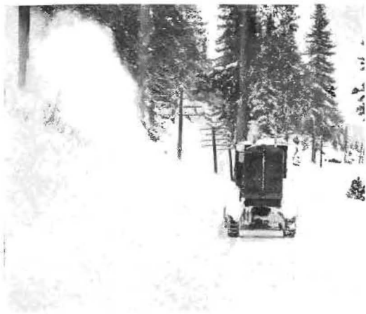
Rear view of auger blower rotary clearing a wide swath through the Donner Summit forests.
