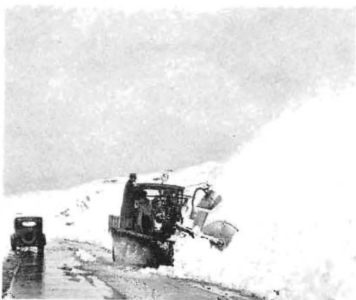
Shovel rotary type truck plow doing its stuff on the Ridge Route near Caswells in Los Angeles County.
