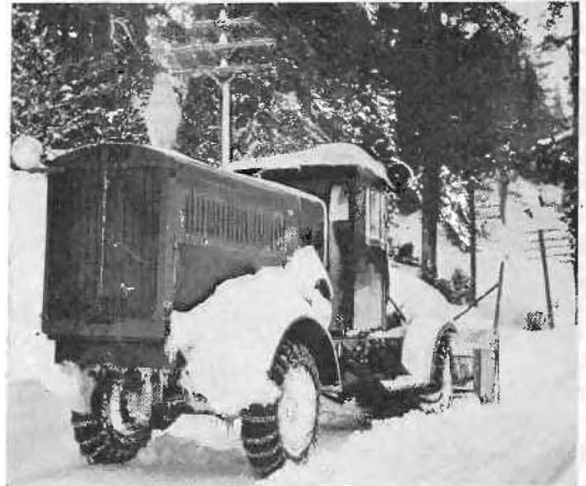
Auger blower type heavy duty plow widening cut through deep drift during storm on the Summit.
