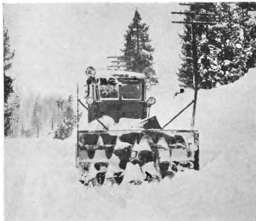
Front view of an auger blower type rotary plow boring its way through the drifts on the Donner Grade.
