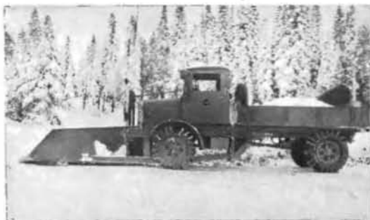
Speed push plow from the Colfax station operating near Soda Springs on the Auburn-Truckee road.
