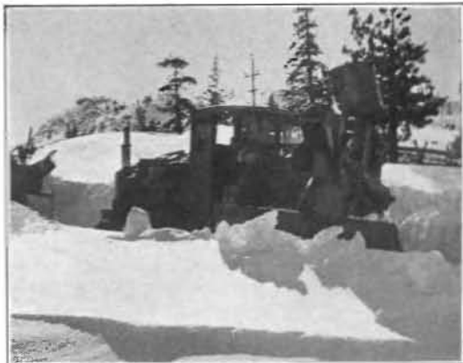
Dual motored four-wheel-drive truck with latest type rotary plow, breaking through plug just west of Donner Summit, February, 1931.
