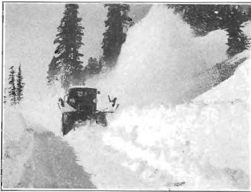
Dual motored four-wheel-drive truck with rotary plow operating east of Soda Springs, near Donner Lake summit, February, 1931.
