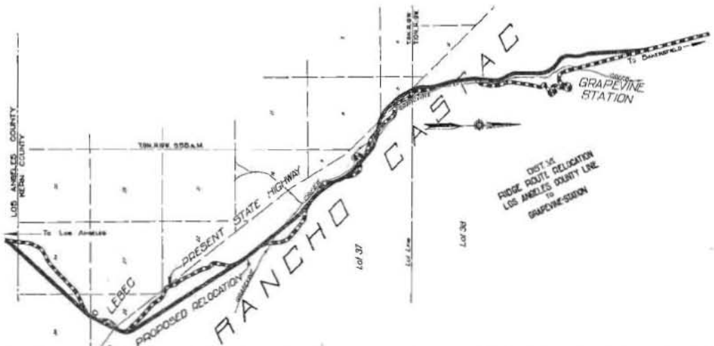
CUTTING CURVES out by the dozen from this Ridge Route unit the relocation of the Grapevine as shown by the diagram will also shorten the distance between Bakersfield and Los Angeles.
